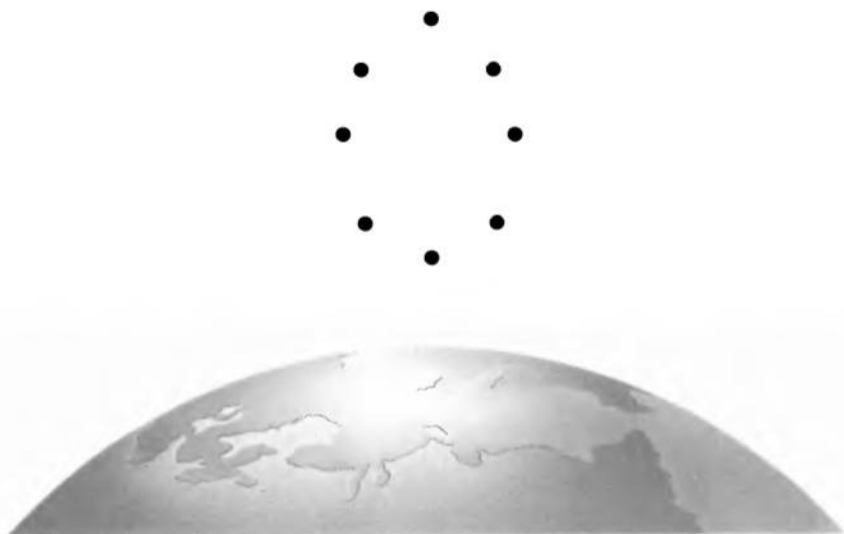
An array of test masses covering the surface of a hollow sphere freely floating above the Earth's surface will shrink in two dimensions and lengthen in one. The volume remains constant; only the shape changes. This change is evidence of the noncontractile, tide-driving spacetime curvature outside Earth.
